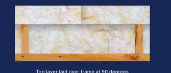
Top layer laid over frame at 90 degrees to bottom (ISIL) layer friction fitted between bottom truss cord.
